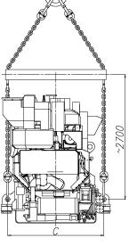
Fig 18-2 Lifting of generating set (DAAE028691D)
