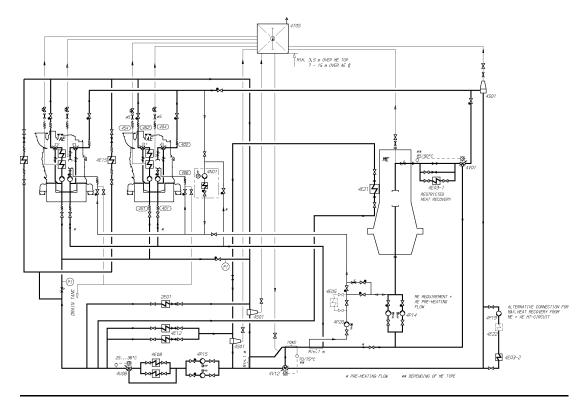
Fig 8-10 Cooling water system, common for ME and AE, mixed LT- and HT-circuit, common heat recovery and preheating for ME and AE (DAAE030653A)
