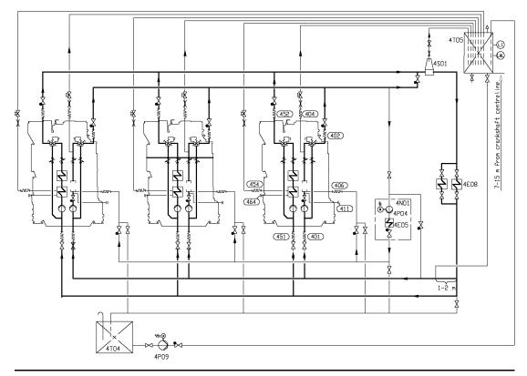
Fig 8-8 Cooling water system, separate system for WA16 engines, without evaporator (DAAF062370A)
