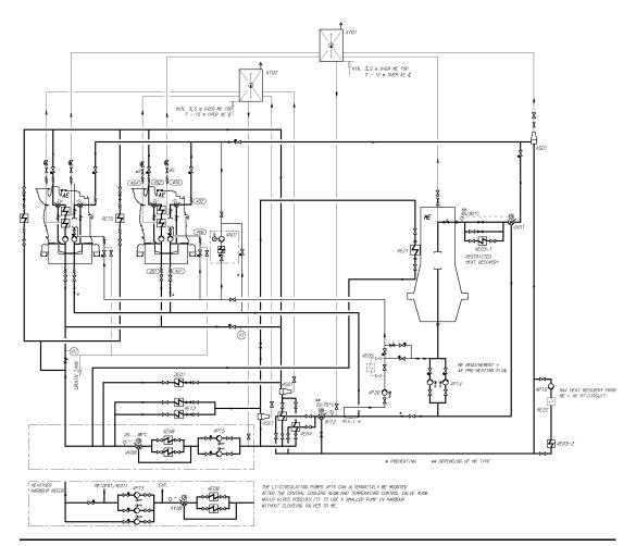
Fig 8-9 Cooling water system, common for ME and AE, split LT- and HT-circuit, common heat recovery and preheating for ME and AE (DAAE030654A)
