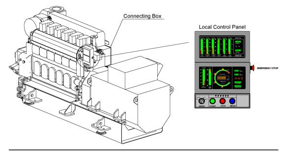
Fig 13-7 Connecting box and Local control panel
