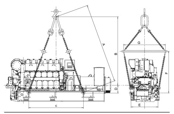
Fig 18-1 Lifting of generating set (DAAT003152C)
