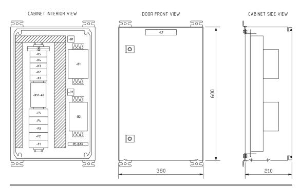
Fig 13-4 Standard power unit (DBAC145268)
