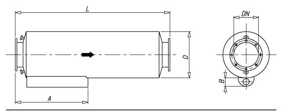
Fig 10-7 Exhaust gas silencer (4V49E0137b)
