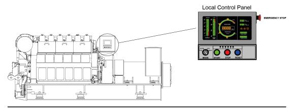
Fig 13-2 Connecting box and Local control panel
