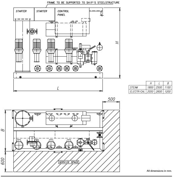
Fig 5-9 Feeder/booster unit, example (DAAE006659)
