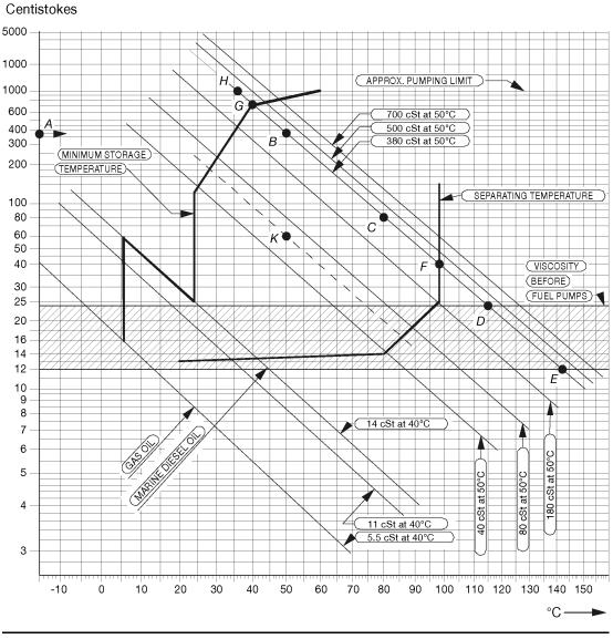
Fig 5-4 Fuel oil viscosity-temperature diagram for determining the pre-heating temperatures of fuel oils (DAAE016379a)
