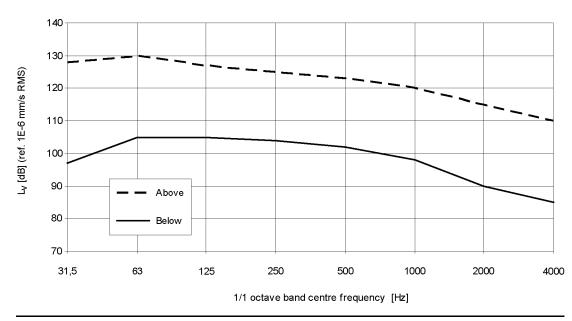
Typical structure borne noise above and below resilient mounts
