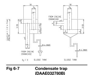
The size of the ventilation pipe (D2) out from the condensate trap should be equal or bigger than the ventilation pipe (D) coming from the engine. For more information about ventilation pipe (D) size, see the external lubricating oil system drawing.
