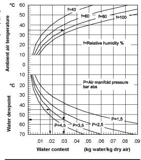
Fig 9-1 Condensation in charge air coolers
