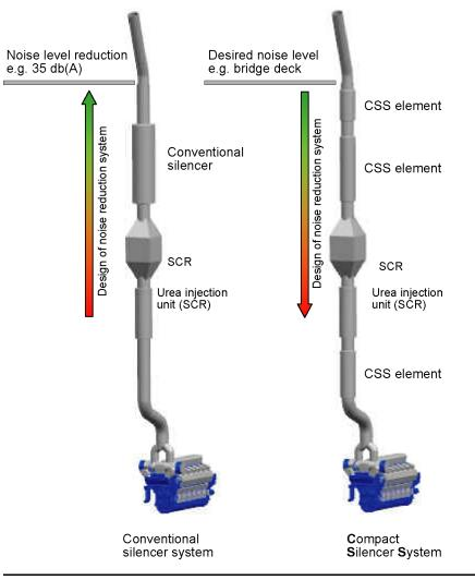
Fig 10-6 Silencer system comparison
