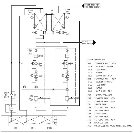
Fig 5-5 Fuel transfer and separating system (V76F6626F)
